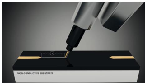
An external alternating electric field causes nanoparticles to assemble in a clearly defined and controlled way to form a line. The process takes place between a stationary and movable electrode.
