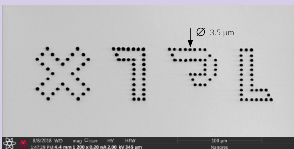
SEM image of XTPL logo pattern composed of microdots deposited on the glass. Dots obtained using technologies available on the market achieve minimum feature size of 20 μm in diameter, while implementing XTPL method allows for depositing dots with the diameter as small as 1 μm.
